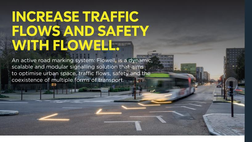
The Flowell solution consists of panels bonded to the pavement that can bear all types of vehicle traffic with the same grip as conventional road surfacing. The panels, composed of LEDs encapsulated in a multilayer substrate, are connected to an electrical grid and controlled remotely.
