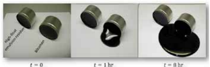
Showing the resistance of high float emulsion residue to flow against C170 bitumen
