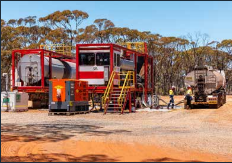
Mobile CRBM blending plant in operation in the Pilbara region
